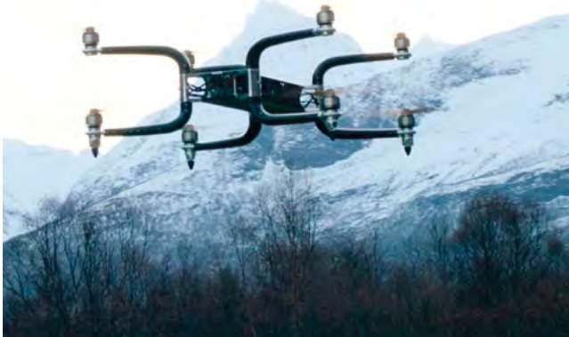
GRIF Aviation 300 - Extra large drone that can carry 500 lbs. Designed with an 8-propeller, the Griff Aviation 300 is the heaviest lift drone that can carry a payload weight of approximately 500 pounds (226 kg) and sustain 31 minutes of flight time. The modular design enables rapid swapping of payloads and batteries in seconds.
