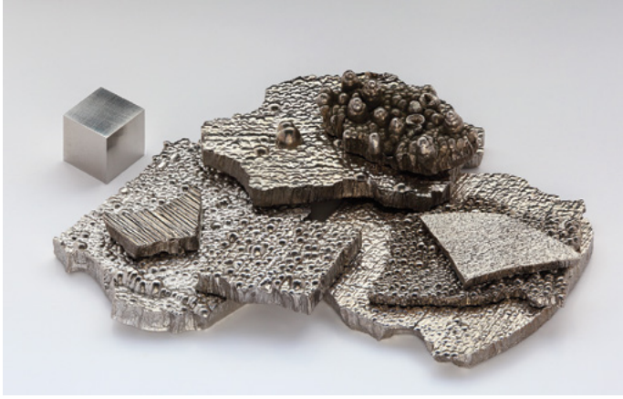
Pure (99.9 %) cobalt chips , electrolytically refined , as well as a high purity (99.8 % = 2N8) 1 cm 3 cobalt cube for comparison. Cobalt By Alchemist-hp (talk- Own work, FAL, CC BY-NC-ND 3.0 )
