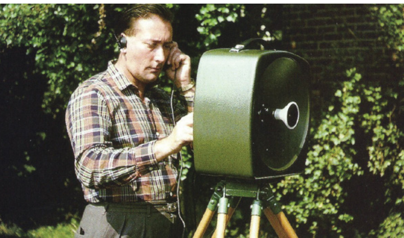
Dr. Alex McEwen had an extraordinary career in surveying, working in 25 countries and in several U.S. states and Canadian provinces. He is seen here operating a microwave distance measuring MRA3 tellurometer.
